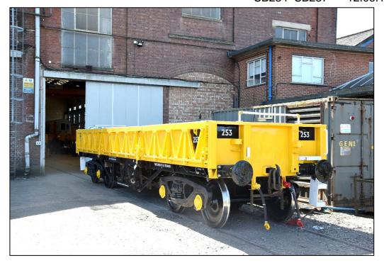
Left: Refurbished Spoil and Ballast Wagon SB253 at Eastleigh on 14 May 2018, looking resplendent after shot-blasting and repainting. A total of 60 ex-BR 4-axle Turbot wagons modified by ABB at Crewe for London Underground. They were built variously by BR at Shildon and Swindon, and RFS at Doncaster between 1982 and 1988. They were delivered to London Underground during January and February 1996. Now, eight are being scrapped and 52 refurbished.
